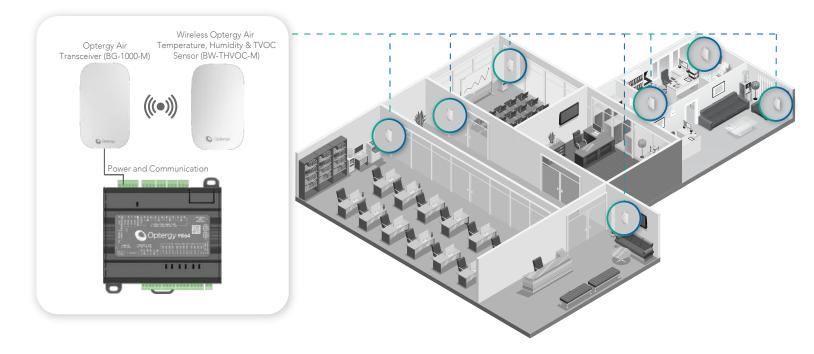
The Optergy Air BW-THVOC-M sensor pairs with the Optergy Air Transceiver (BG-1000-M). Up to seven (7) Optergy Air BW-THVOC-M sensors can be connected to one Optergy Air Transceiver (BG-1000-M).
