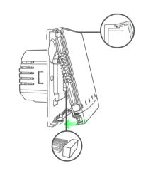
Surface mounting in a 60mm wall box. Make sure the back cover is in the appropriate position (according to the arrow on it)
