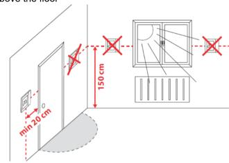
Devices must be mounted on clean, dry indoor place without direct airflow from a heating / cooling device, and not be exposed to dripping or splashing
