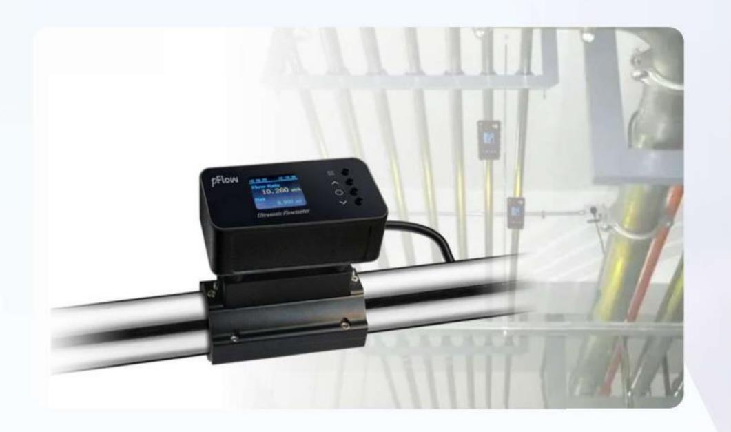
Gentos quick measure ultrasonic flow meter F3CL\F3RO adopts the ultrasonic transit time measurement principle, combined with Gentos patented flow algorithm technology, it realizes accurate measurement of the fluid flow in the pipe. The product is all-in-one and clip-on structure design, which is simple and convenient to install. Only four steps are needed all along. The installation process requires no contact with fluid media and no need to shut down.
