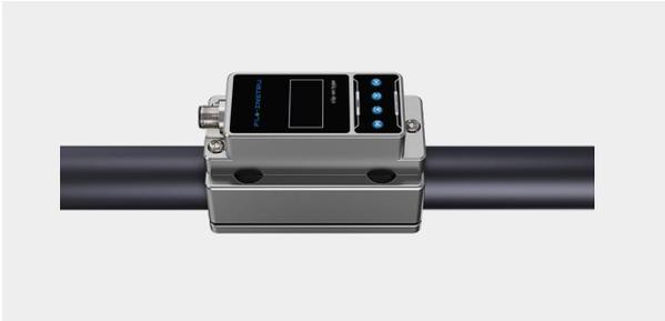
Remove the protection film outside the sensor, put the sensor part into the bracket, and fasten the two M4 screws.
