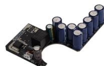
\*Failsafe via internal super capacitor
