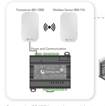
One transceiver (BG-1000) is required per one wireless temperature and humidity sensor (BW-TH). The BW-TH uses a BG-1000 to connect to an Optergy P864. Its datapoints then belong to the connected Optergy P864.
