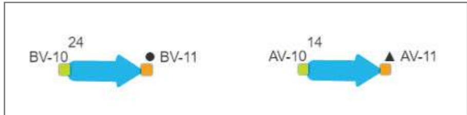
**Note:** Values that are negated will appear with a solid dot above the input or output for binary values and a solid triangle above the input or output for Analog Values.
