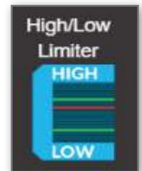
The output will equal the analog input as long as it is within the range defined by the high limit and low limit.
