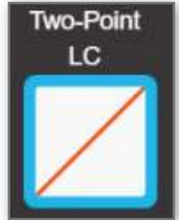
A straight-line relationship (of the form  $y = a + bx$ ) determines the output as a function of the input.
