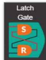
A minimum of 1 program cycle is required on the set (S) input is required to be True (1) and the Reset (R) input is False (0) to set the output to True (1).
