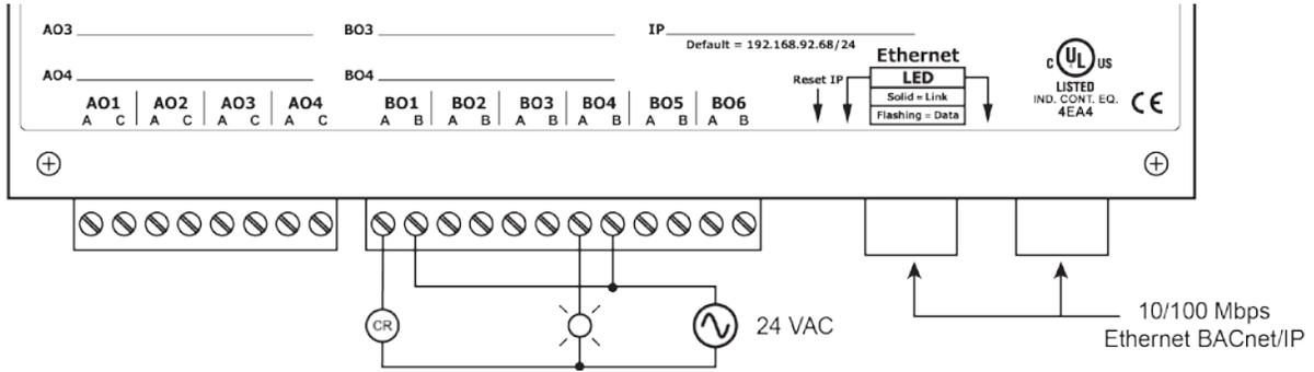
**Figure 9 — Binary Output Connections**
