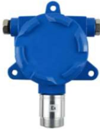
This ammonia detector has electrochemical sensor to detect  $\text{NH}_3$  gas concentration in air by natural diffusion. Sensor produced in UK with good sensitivity and repeatability. It is with explosion proof shell, IP65 water and dust proof. Collects and transmits the data to the controller through 4~20mA or RS485 Modbus in real time. With an optional audible & visual alarm light, when the gas concentration exceeds a preset alarm point, it will make alarm immediately.
