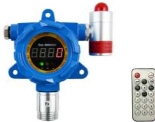
This ammonia detector is with electrochemical sensor to detect NH<sub>3</sub> gas concentration in air, sensor produced in UK with good sensitivity and repeatability. It is with explosion proof shell, IP65 water and dust proof. Collects and transmits the data to the controller through 4~20mA or RS485 Modbus in real time. With an optional audible & visual alarm light, when the gas concentration exceeds a preset alarm point, it will make alarm immediately.
