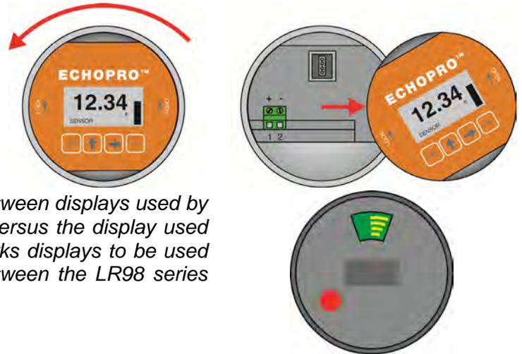
**Note:** *There is an internal configuration difference between displays used by the EchoPro® sensors (LR36, LR41 & LR46 series) versus the display used with the LR98 series. A colored dot on the back marks displays to be used only with the LR98 series. Never swap displays between the LR98 series and other EchoPro® sensors.*
