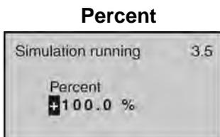
This method uses percentage of span (0-100%) to set the current output (4-20mA) between the Empty and Full Configuration values with 100% equal to 20 mA and 0% equal to 4mA.
