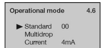
This function allows for the loop consumption (constant current draw) to be set to either 4mA or 8mA. **Default is 4mA.**
