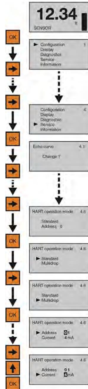
When the setting is correct for your application, press **Enter** again to return to HART® Operational Mode, press the **ESC** button to return to Service Menu and press **ESC** a second time to return to the Main screen.
