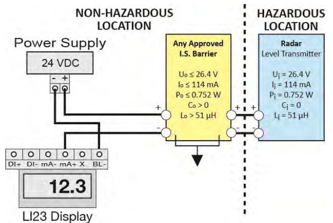
**Note:** Always refer to the Control Drawing 301901 for further wiring information.
