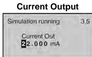
This method directly sets the current output (4-20mA) to the desired value.
