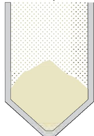
**SOLIDS WITH LARGE ANGLE OF REPOSE**
