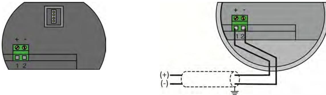
The sensor should be wired with shielded 2-conductor cable (16 to 22 AWG) to protect from electromagnetic interference. If using a liquid tight connector, select a cable with an outer diameter that is designed to ensure an effective seal with the connector [typically between 0.20" to 0.35" (5 to 9 mm)].
