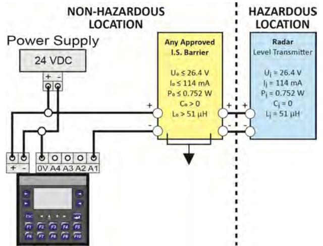
**Note:** Always refer to the Control Drawing 301901 for further wiring information.
