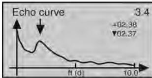
First Echo peak is normal and no adjustment is required.
