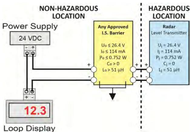
**Note:** Always refer to the Control Drawing 301901 for further wiring information.
