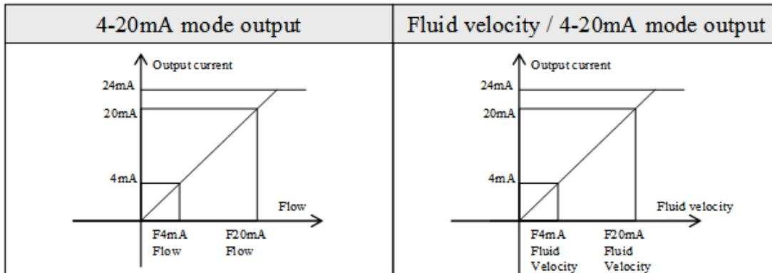
In two graphs shown above, flow  $F_{4mA}$  indicates the value that the user entered in Window M57; and flow  $F_{20mA}$  indicates the value that the user entered in Window M58. In the 4-20mA modes,  $F_{4mA}$  and  $F_{20mA}$  can be selected as a positive or negative flow value as long as the two values are not the same.
