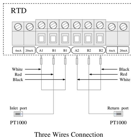
The two PT1000 temperature sensors are installed on the inlet and return pipes and they will input temperature signals to the D116 transmitter.
