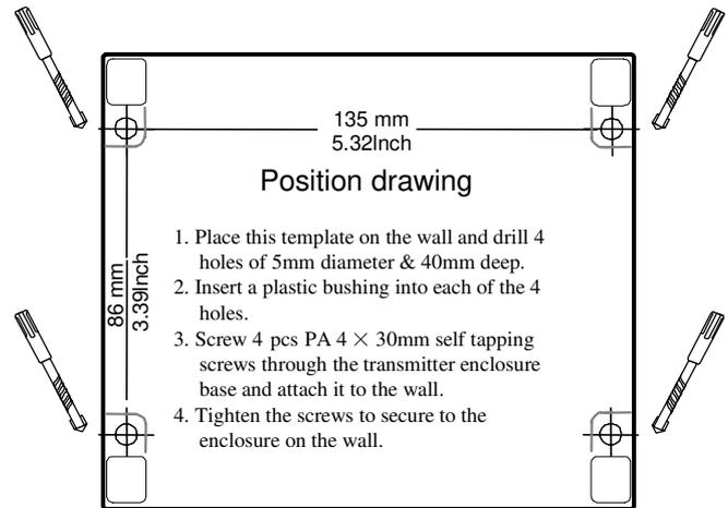
Take out the enclosed screws and plastic bushings. Insert the plastic bushings into the installing holes. Put the flowmeter to the position and screw it in.
