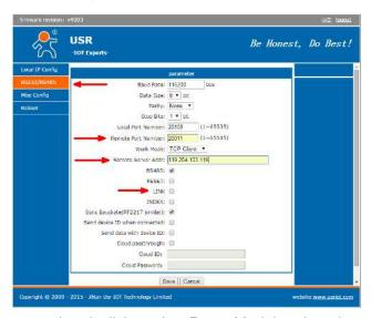
3.4 Set up completed, click on the "Reset Module", then the system will pop up the prompt of set up successfully.
