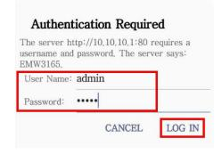
5. At this point, get into the WIFI module Settings interface. We will need to modify the parameters setting. The majority changes concentrate in "Wifi Mode Select", "Station Mode Setting" and "Network Setting".
