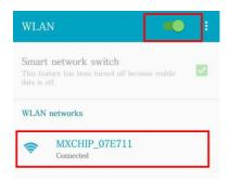
Note: researched WIFI hotspot is like MXCHIP\_07E711, MXCHIP\_ is an invariant format, 07E711 is a unique serial number for a WIFI module. Different WIFI modules have different serial numbers. It will be shown on the surface of the WIFI module.
