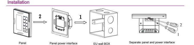
Installation: Hold the edge of the panel (shown as above), insert the power interface module vertically. Do not push the panel too hard.
