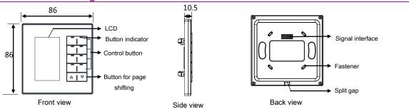
Button Indicator: Indicates the status of the target. On-Status on, Off-Status off.
