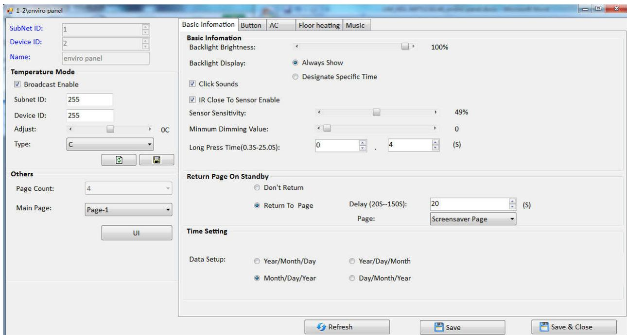
**Temperature Mode:** This panel built-in temperature sensor, can broadcast the temperature to the BUS. If the detected temperature has error, you can adjust it on the software.
